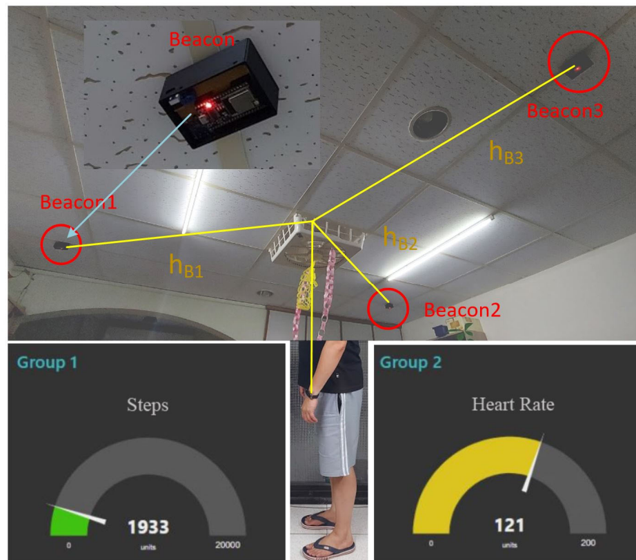
Figure 11. The position of each beacon device on the ceiling.
