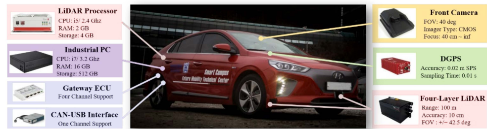
Figure 2. Configuration of the data collection vehicle. Adapted from ref. [45].
