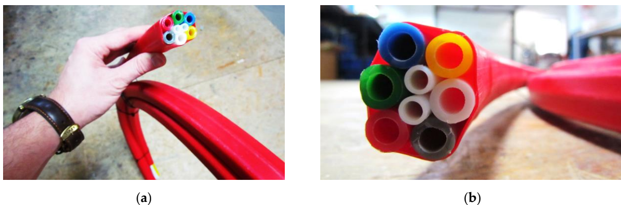
Figure 6. Prototype version of new hydraulic sensor SHM Profiler: (a) general view; (b) close-up to the cross section.
