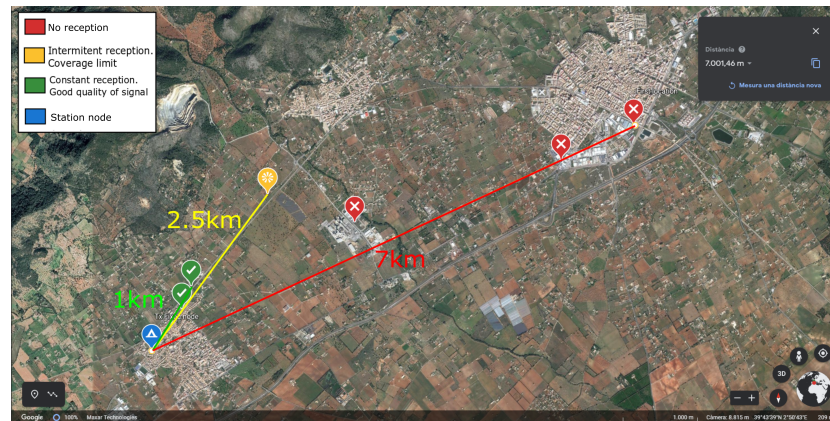
Figure 11. Experimental coverage test in an urban area, performed between Inca and Binissalem (Mallorca, Spain).
