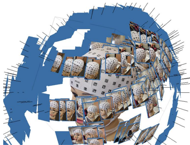
Figure 12. Final photogrammetric exterior orientation (alignment) used to create the 3D model presented in Figure 10. The black lines represent the camera’s projection center, and the blue areas represent the photography coverage area.
