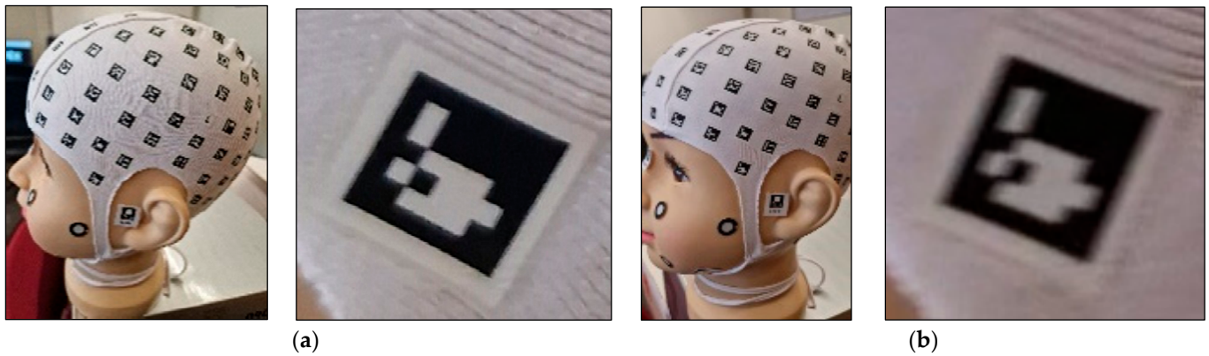
Figure 9. Comparison of input images: (a) Zoom in of an image obtained with the camera (4000 × 3000 pix); (b) Zoom in of an image obtained with the video (1080 × 1920 pix).
