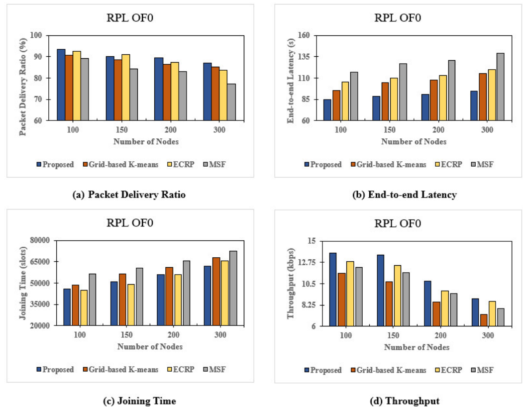
Figure 9. Graphs showing results for the Objective Function Zero (OF0) routing protocol: (a) Packet Delivery Ratio (PDR), (b) end-to-end latency, (c) joining time, and (d) throughput.
