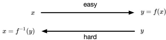
**Figure 1.5** The general concept of a one-way function.
