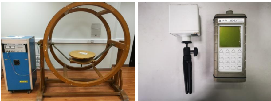
Figure 7. Power-frequency Magnetic Field Experimental Equipment(left) and Teslameter and Standard Probe(right).
