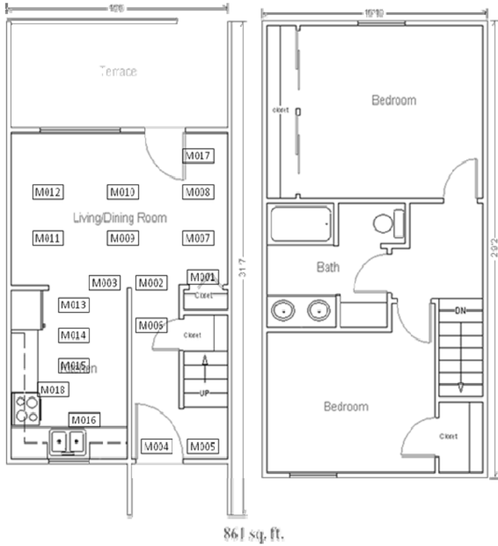
Fig. 2. WSU Tulum smart apartment testbed and motion sensor layout.
