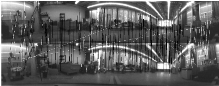
Figure 16. Landmark matches: Black: valid matches, white: rejected outliers.
