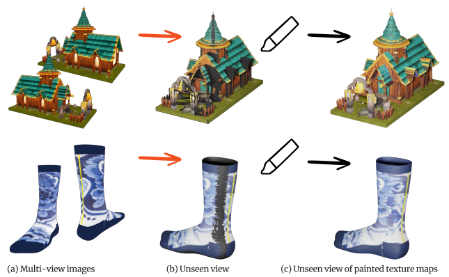
Fig. 9. Texture completion from sparse views. With sparse views of objects provided (front and back views as shown in (a)), unprojected textures retain many unseen regions (b). TEXGen effectively fills these unseen regions with harmonious textures (c).
