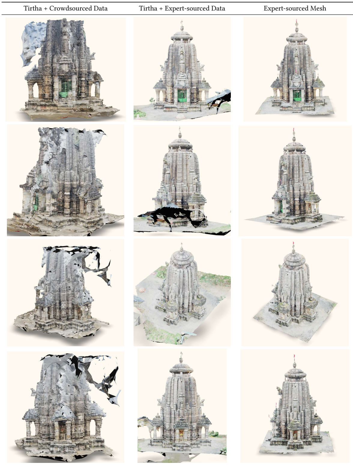
Figure 8: Gopinatha Temple: Comparing the level of detail between Tirtha’s and Metashape’s reconstructions
