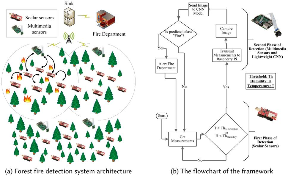
Fig. 1. Forest fire detection system architecture and information flow chart for first and second phase of detection.
