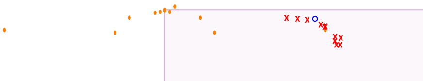
Figure 5: Graphical representation of the dimer problem. The orange points are the 12 poles of the rational function. The shaded part is the region used in the NLEIGS solver, while the blue circle is the target value used in NLEIGS as well as the other solvers. Red crosses are the 20 eigenvalues computed by NLEIGS (there are more eigenvalues inside the region, and other solvers may not return exactly the same ones).
