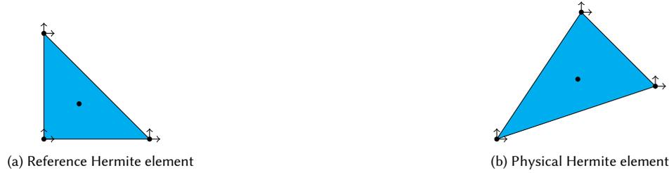
Fig. 4. Reference and physical cubic Hermite elements with gradient degrees of freedom expressed in terms of local Cartesian directional derivatives.
