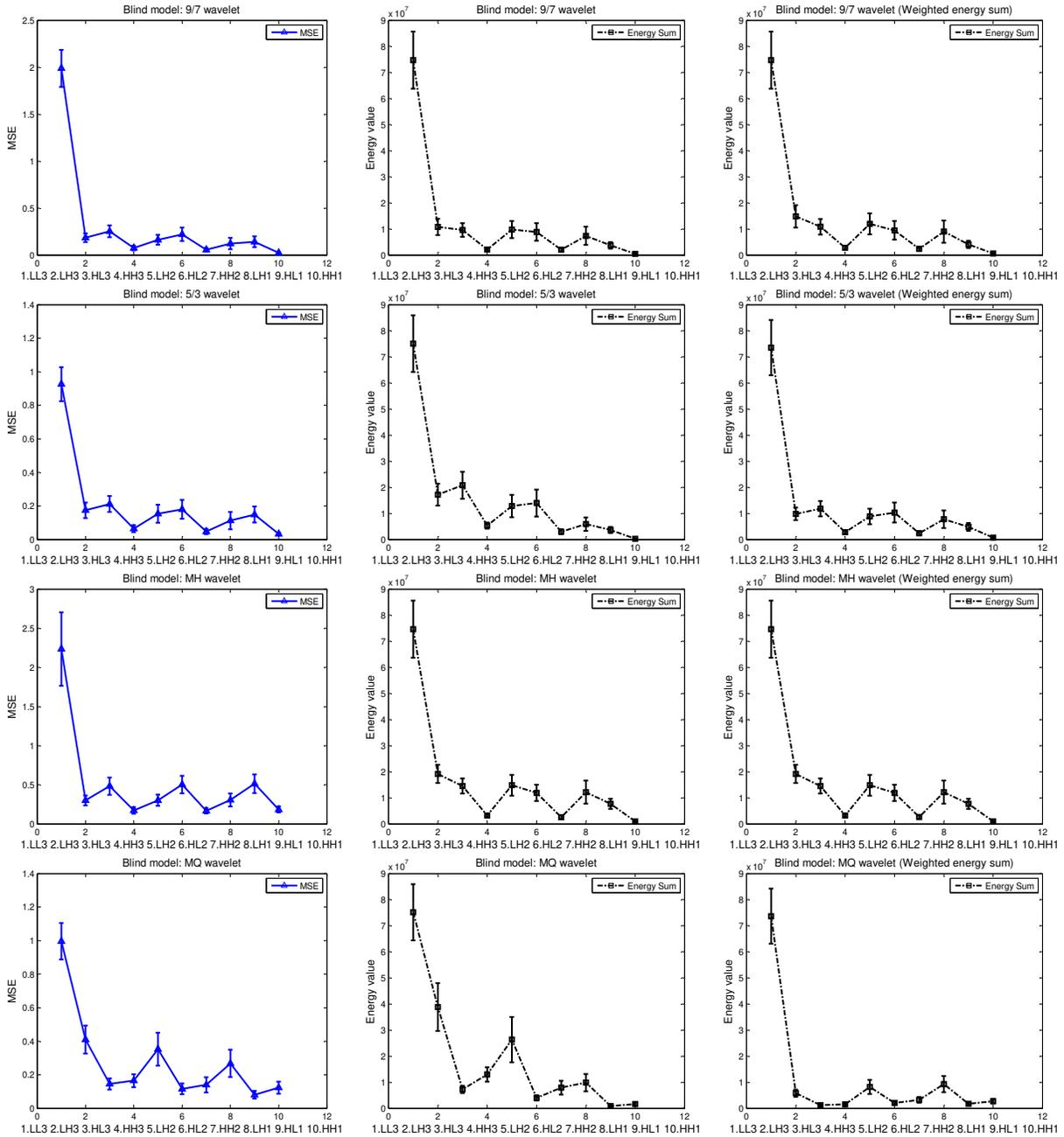
Fig. 9. Watermark embedding (blind) performance graph for various wavelets in different subband. Wavelet kernels are shown top to bottom as 1. 9/7, 2. 5/3, 3. MH and 4. MQ, respectively. *Column 1, column 2 and column 3* represent the MSE, energy sum without and with weighting parameters, respectively.
