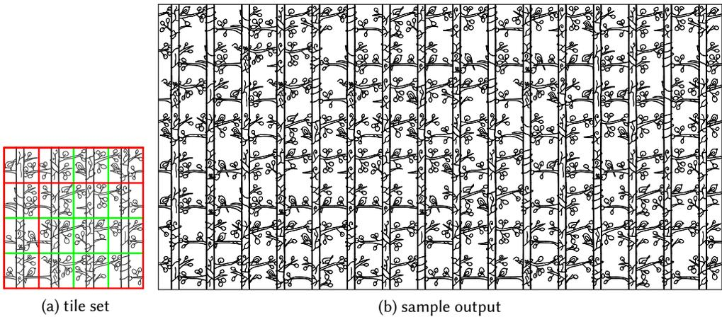
Fig. 1. Tile-based pattern design. Users create a tile-set (a) with desired appearance and structure via our authoring interface. From (a), our synthesis method can quickly tile outputs with designated sizes and shapes (b) and suitable for digital manufacturing (Figure 2a).
