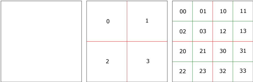
Fig. 5. Hierarchical tiling process. Starting from an output domain (left), we first divide it into 4 quadrants and synthesize them in the order as indicated by the numbers (middle). We can repeat this process recursively for another level (right) until each subdivided tile has small enough size for basic tiling.
