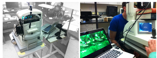
Fig. 4. Overview of the autorefractor setup. Back view (left) and subject measurement (right).
