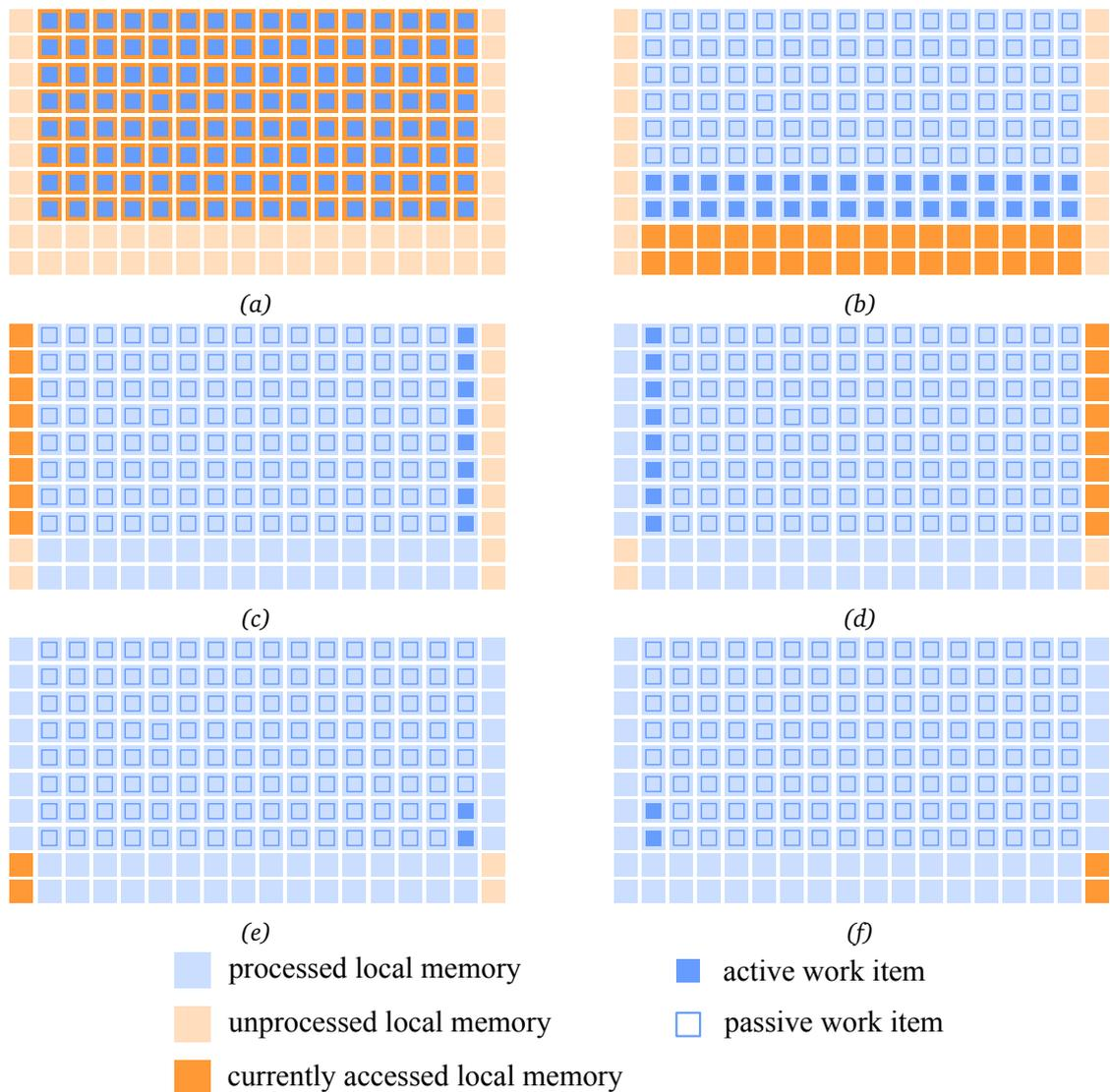
Figure 7.7: Outline of an efficient pattern to load a region of local memory using the work items that are required for a stencil computation. The size of the work group is  $[16,8]$  and the region of the local memory is  $[18,10]$ . Steps (a) through (f) illustrate the access pattern that is used to load the memory.
