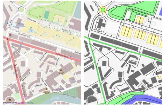
Figure 5: An OpenStreetMap map excerpt of Edinburgh comparing a rendering from OSM ( left ) and one using our own rendering, which is based on line and area features ( right ).
