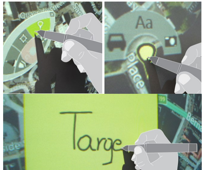
Figure 3: The tool palette ( top left ) for placing textual annotations ( top right ) or drawing sketched content on the map ( bottom ).
