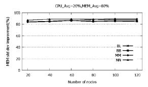
Figure 5. Balancing effect of policies on Memory when avg. (CPU, MEM) loads are (20%, 80%)
