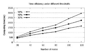
Figure 13. NN time efficiency under different thresholds
