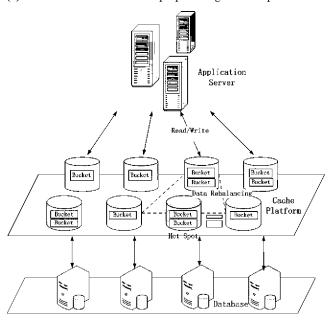
Figure 1. Scenario of Load Balancing in Cache Platform
