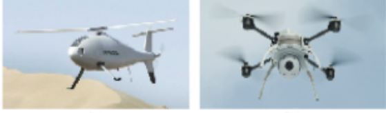
Figure 3: Examples of possible UAVs: (Left) Schiebel Camcopter 1 S-100, which can stay airborne for more than 6 hours with an operational range of 45km to 180km and costs approximately $500,000; and (Right) Aeryon Labs Inc. Scout, which can stay airborne for up to 25 minutes with an operational range of 25km and costs approximately $50,000.
