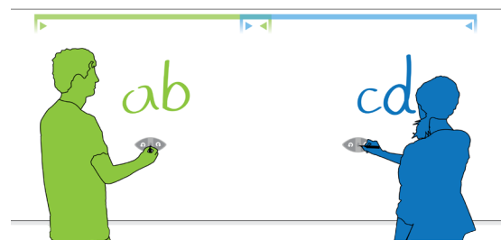
Figure 11: In our implementation, workspaces are visualized by color-coded bars on top of the screen. Inward arrows clarify overlapping workspaces. Positioning the bars at the top of the workspace limits the visual clutter during work.
