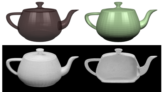
Figure 7: The top left image shows a polygonized version the Utah teapot which contains holes (around lid and tip of spout), and intersecting parts (handle and spout with body). The top right image is a near-interpolating surface which fills the holes and removes intersecting surfaces. The bottom row contains photographs of physical models built on a fused deposition machine. The bottom right image shows a physical cutaway model.
