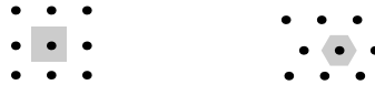
Figure 4: (a) The figure on the left shows that the Voronoi region about a point in the square lattice L_S is given by a square of unit length; a tile K in the plane obtained by a union of unit squares about points in L_S is called a quasi-polyomino. (b) A Voronoi region about a point in the hexagonal lattice L_H is a hexagon; a tile K in the plane obtained from a union of these Voronoi-hexagons about points in L_H is called a quasi-polyhex.
