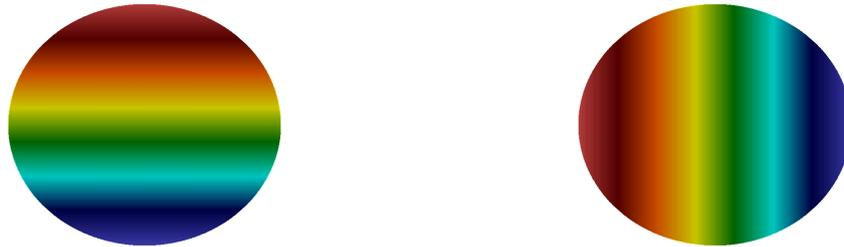
Figure 4:  $x$ -component (left) and  $y$ -component (right) of the eigenfunction  $\mathbf{u}_{h,1}$  on the unit disk associated to the eigenvalue  $\kappa_1 = 0$ . The computations are performed on a grid comprising of triangles.
