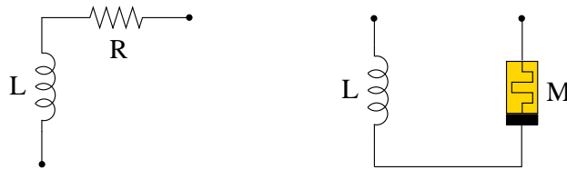
Figure 2: L-proper trees in the circuit of Figure 1
