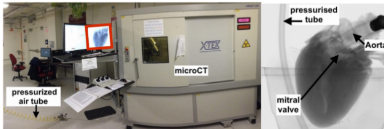
Figure 2. Data acquisition : Micro CT device with pressurized air tube going inside and its screen (in red and zoomed on the right) displaying an Xray of the porcine heart.
