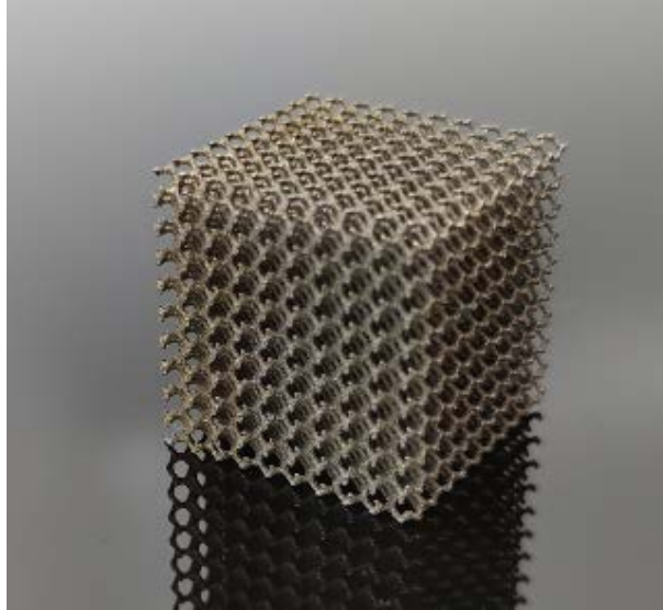
FIGURE 2: Ti6AL4V bone scaffold composed of gyroid structures
