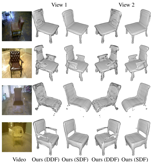
Figure 6. Qualitative results of 3D reconstruction from 40 real-world videos of chairs from Redwood dataset [11]. We reconstruct chairs by optimizing for photometric consistency between different frames of videos using the depth predicted by our model. Left: A frame from the input video. Right: DDF renders and reconstructed SDF in two views. The average distance from the predicted shape to the ground truth mesh is 4.0cm.
