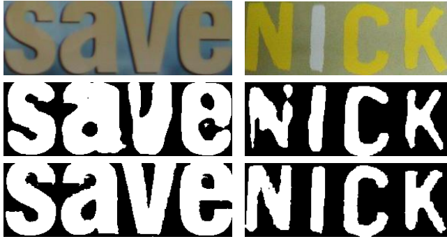
Figure 4. The first row is input images, second row is raw FCN predictions and last row contains final results with CRF refinement.
