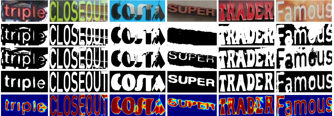
Figure 6. In this figure we compare the result of Otsu binarization algorithm [28], Zhou’s text segmentation algorithm [42] and our method with several challenging images. From top to bottom: input image, Otsu result, Zhou’s result, our result and our raw FCN output probability map.
