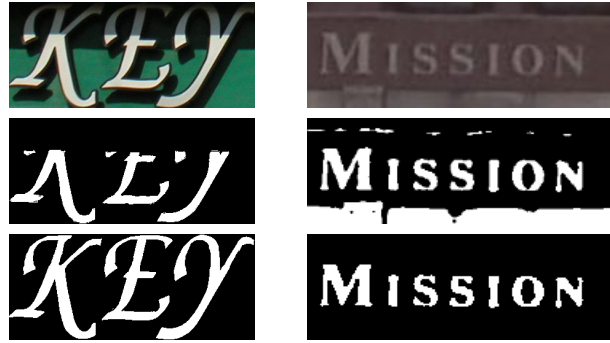
Figure 5. The first row is input images, second row is results without stroke width kernel and last row contains results with stroke width kernel. In left example the text color has large variance due to shadow and for right image the background contains regions with similar color as text region. In these cases use bilateral kernel alone becomes unreliable.
