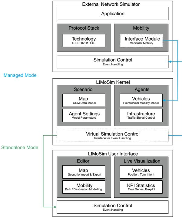
Fig. 3. Components of the proposed LIMoSim. The simulator can either operate in *managed* mode, where an external network simulator takes control about the event handling mechanisms or in *standalone* mode using an optional user interface. As opposed to the IPC-based approach, the coupling is realized by direct code references and does not require a dedicated protocol.
