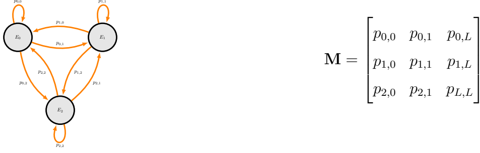
Figure 1. The state transition diagram and the corresponding transition probability matrix of the Markov chain, in the case of L = 2 .
