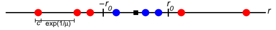
Fig. 1. The vehicles are modeled as identical impenetrable disks. The vehicles outside of the cell (red disks) generate interference to the base station (black square). The rest (blue disks) are paired with the base station. In the figure, the tracking distance is illustrated equal to the diameter of the disk.
