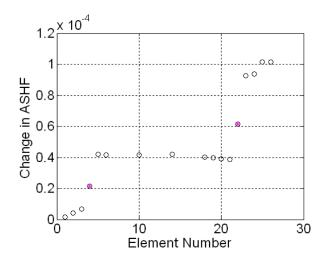
Figure 3: Example ASHFM damage indicator output; shaded dots correspond to damaged elements
