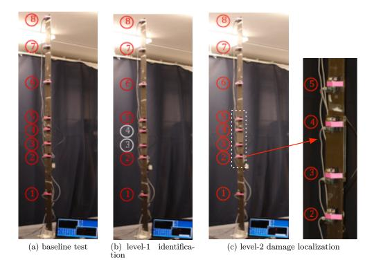
Figure 6: The cantilever beam and sensor placements for each stage of the experiment
