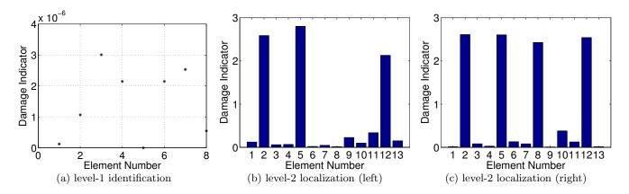
Figure 8: Damage localization results on the simulated truss
