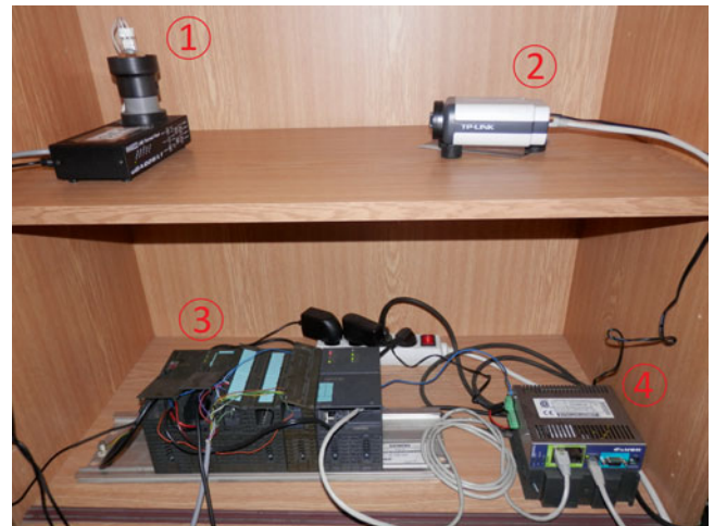
Fig. 6. Devices in remote lab physical setup: ① controlled experiment (thermo-optical plant uDAQ28/LT), ② IP camera, ③ PLC Siemens S7-300, ④ INR device eWON4005CD.
