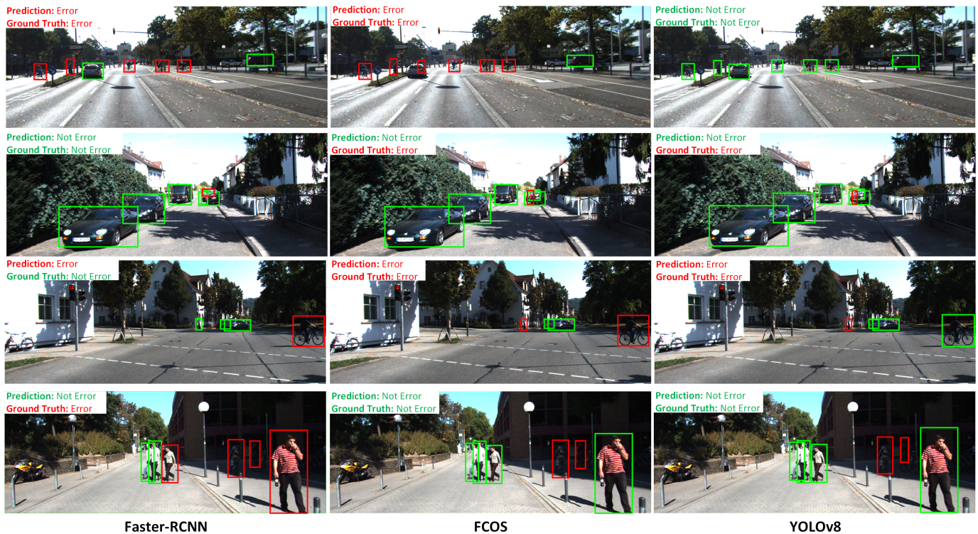
Fig. 7. This figure presents the introspection mechanism’s performance variations across three distinct object detection models—Faster R-CNN (left column), FCOS (middle), and YOLOv8 (right) — each represented by a separate column, applied to the same urban street scenes taken from KITTI dataset. While the occurrence of missed objects and the resultant error labels may vary between detectors, a degree of similarity is observed among one-stage detectors like FCOS and YOLOv8. Annotations highlight the correct and incorrect predictions of the object detection functionality: red boxes indicate false positives or false negatives, indicating detection errors, whereas green boxes denote true positives. A sample is categorised as ‘non-error’ in the error dataset if its mean Average Precision (mAP) surpasses the set threshold, and ‘error’ if it does not. The introspection model’s predictions, along with the ground truth, are detailed in the upper left corner of each image, enhancing the understanding of each model’s detection capabilities and the introspection’s result.
