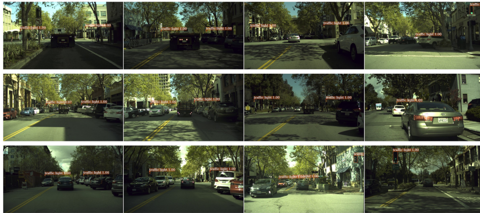
Fig. 9. Example detection results on the Bosch Small Traffic Lights test set. See Section IV-B for details. Best viewed electronically, zoomed in.
