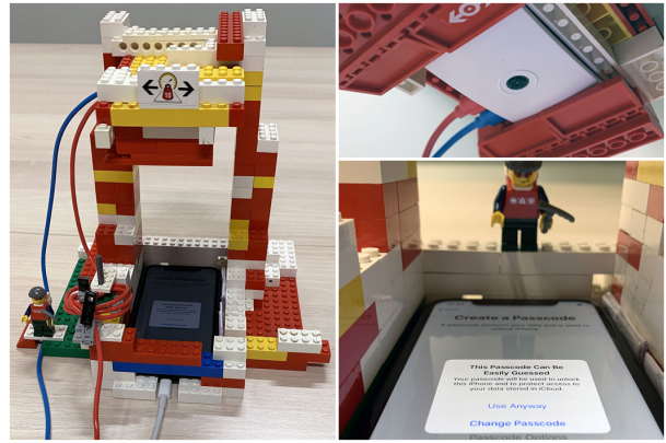
Fig. 1. The installation used to extract the iOS blocklists.
