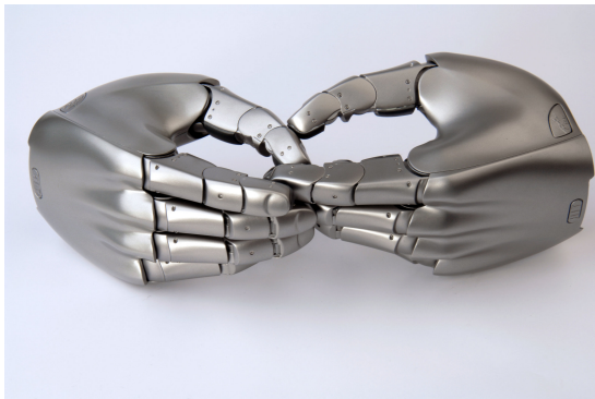
Fig. 1. 5-fingered dexterous robot hand DLR-HIT-hand II
