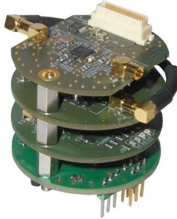
Fig. 6.1: The IHPstack a "Lego-like" sensor node for low power sensor applications, the platform for langOS, a highly configurable sensor node OS library.
