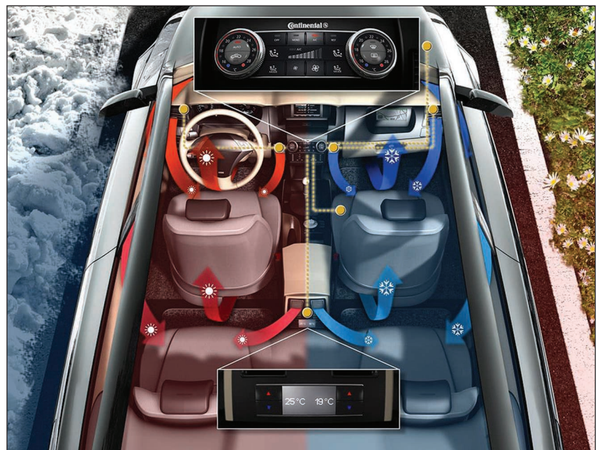
FIGURE 7 HVAC control. (Source: https://conti-engineering.com/ ; used with permission.)
