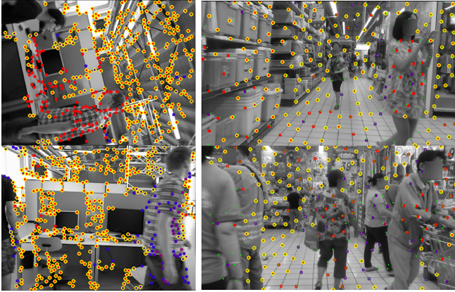
Fig. 7. Results of Moving Consistency Check. Features without yellow circular are the outliers marked by the Moving Consistency Check module.
