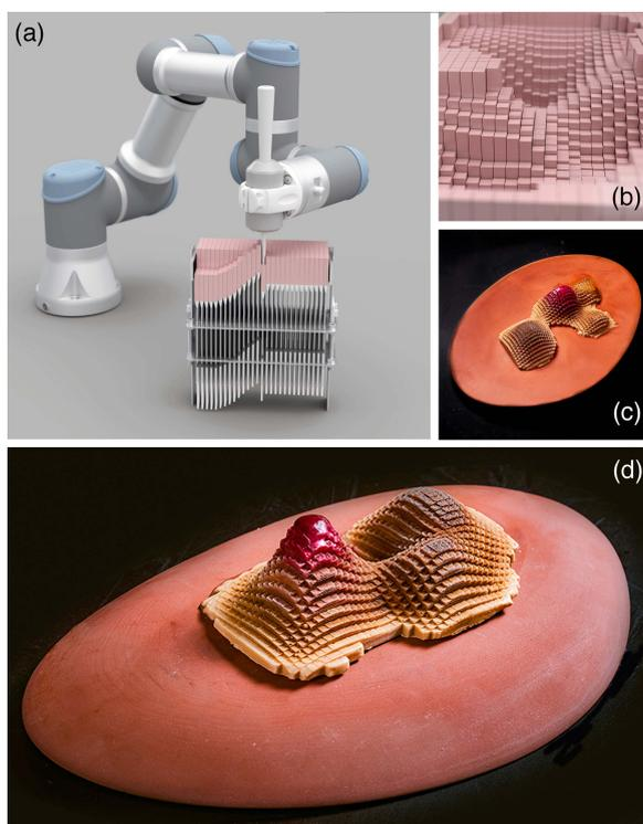
**Fig. 4.** (a) Illustration of a robot arm modifying a programmable silicon mold. (b) Mold. (c) and (d) Two versions of a mousse dessert, exemplifying the potential of the modular mold.
