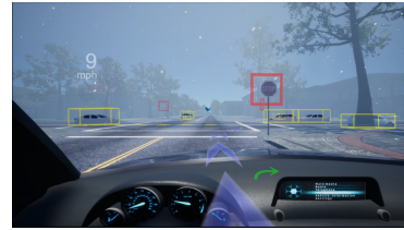
Fig. 1. An example screenshot of the study scenario of low visibility and high automation transparency. The bounding boxes highlight the signs, cars and other moving objects in sight.
