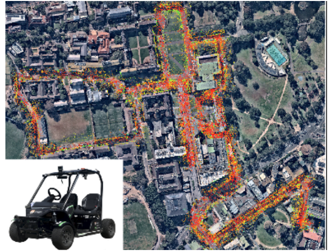
Fig. 1. The lidar point clouds superimposed and projected on horizontal plane as a layer in GIS is precisely registered and overlaid onto high resolution orthogonal aerial imagery. The dataset was taken by an electric vehicle starting from bottom right corner, driving through the University of Sydney main campus in multiple loops, and back to the starting location. The electric vehicle is equipped with Velodyne VLP 16 beam lidar and multiple sensors
