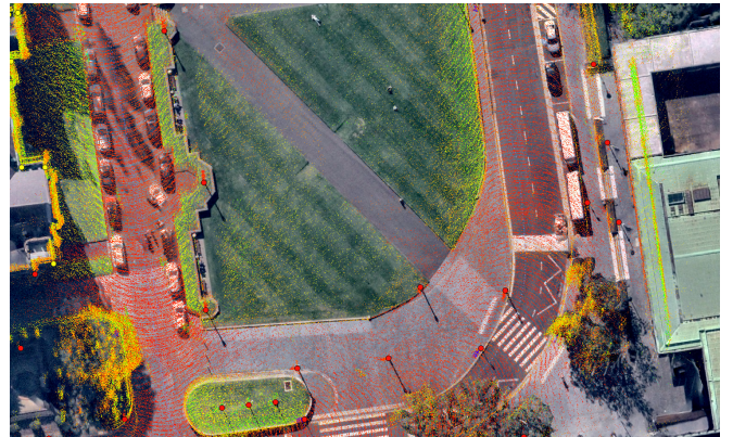
Fig. 10. Close up look of accurately registered lidar orthoimage. Inaccuracies are mainly in longitudinal direction and when vehicle turning corners. Colors represent reflectivity.
