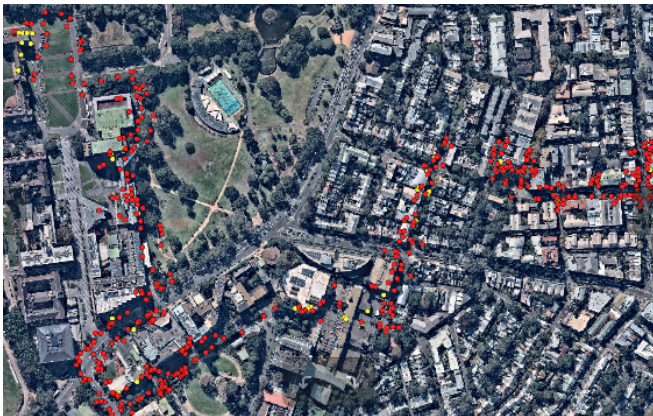
Fig. 4. Resulting landmark map from method IV-B overlaid on aerial map in GIS. Drifts are corrected and landmark positions follow road networks. The improvement is more noticeable at the beginning and end of the run when compared with previous approach.
