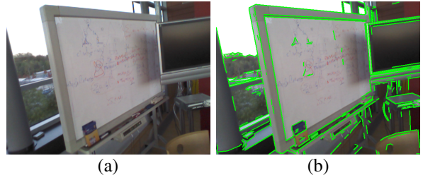
Fig. 1: Line segment example. (a) Input image (b) Line segments. In scenes with little texture and repetitive patterns which are typical in indoor environments, line segments are more robust.
