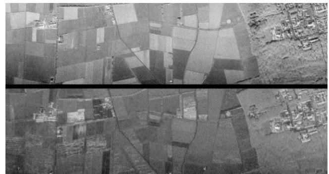
Figure 3: Example of processed SAR data (HH) simultaneously acquired during the Sarsense campaign. Top: L-band, bottom: C-band.
