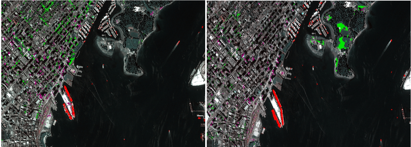
Fig. 4: Change Detection from multitemporal, multi-sensor between: (a) a Deimos March'15 and a Deimos May'15 ( DI-D2 , left), (b) an Iris video sequence (first frame) and a Deimos May'15 ( V-D2 , right).
