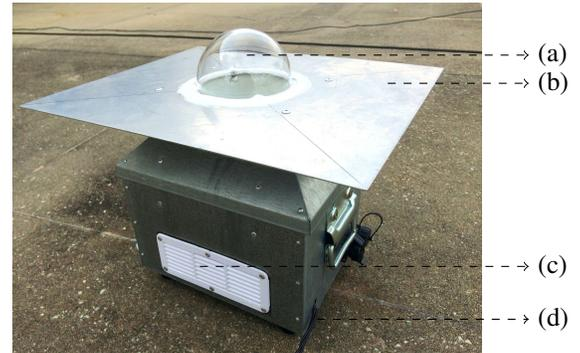
**Fig. 2:** Ventilated WAHRIS design. (a) Dome, (b) shelter, (c) air vent cover, (d) casing.
